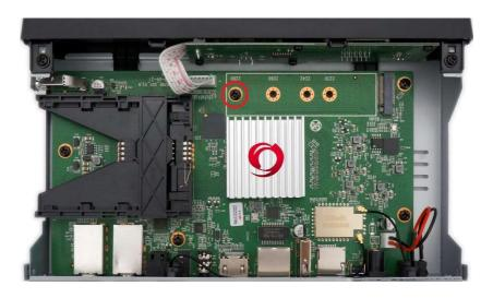
Insert the M. 2 SSD at a 30-degree angle into the appropriate slot. Press the
